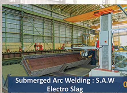
03 Submerged Arc Welding : S.A.W
